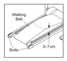
turn both rear roller adjustment bolts counterclockwise 1/4 of a turn. When the tension of the walking belt is correct, you should be able to lift each side of the walking belt 5 to 7 cm (2 to 3 in.). Walk on the treadmill for a few minutes. Repeat until the walking belt is properly tightened. Be careful to keep the walking belt centred.
